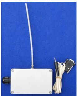
The transmit / receive range of Active Tags with the ADS / PDS - fixed unit is between 5 and 30 meters in diameter. The range is adjustable on the reader & is also dependant on screening by Metal.
